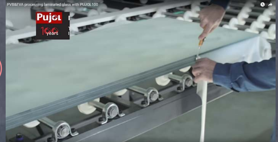
The extra VAC (PVB film) on the sides were cut and discarded
